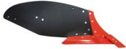
MP4WP - Full mouldboard, semi-helical, ideal for very sticky soils. (Working depth 20-30 cm).
