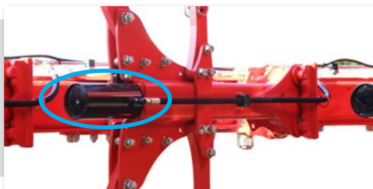
1st and 4th body with increased cylinder bore.
