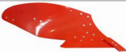
MP4WN - Full mouldboard, semi-helical, ideal for heavy/humid soils. (Working depth 20-30 cm).
